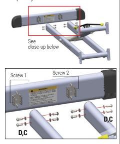
**STEP 7.** Lay the Recovery Series LEX on its side. Using the hardware (C, E) as indicated; attach the Rear Struts / Incline Strut as shown. Tighten completely.
