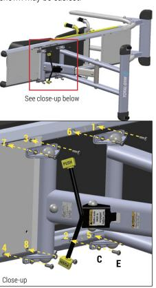
**STEP 8.** Turn the LEX upright and, using the hardware (H, J, K, S) as indicated; attach the Squat Stand to the Struts. Tighten completely. Installing the screws in the order shown may be easiest. Once screws are fully tightened, push on all 12 caps (S).
