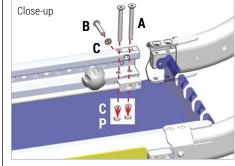
**STEP 4.** Install the hardware (G, F) on both rails as shown below.
