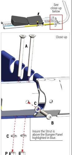
**STEP 3.** Repeat STEP 2 on other side, attaching the Right Squat Strut to the Right Rail using the hardware (A, B, C, P) as shown, but do not tighten completely.
