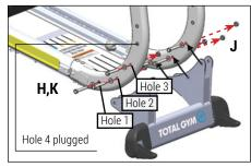
The image below is how the Front Base attached to the Struts should look.
