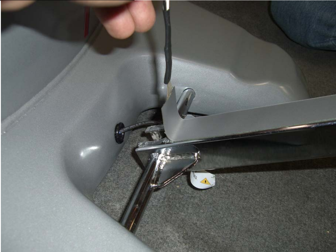
Pull the switch off by the wires from the bottom near the tower toward the rails
